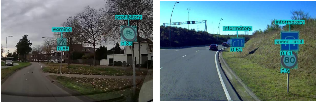
Figure 10: Inference examples from the trained traffic sign detector on out-of-distribution data from the Netherlands.
