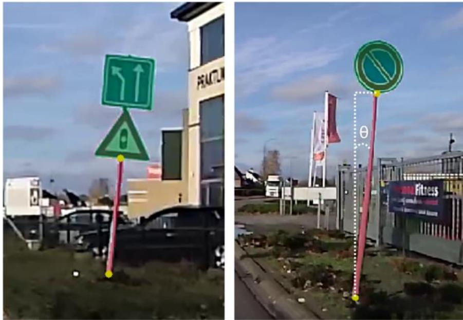
Figure 11: Example of skew calculation for two traffic signs. The predicted segmentation masks for the traffic sign board and corresponding pole are shown in green and red, respectively. In the right image, the skew is given as the angle \theta and indicated using the white dotted lines.
