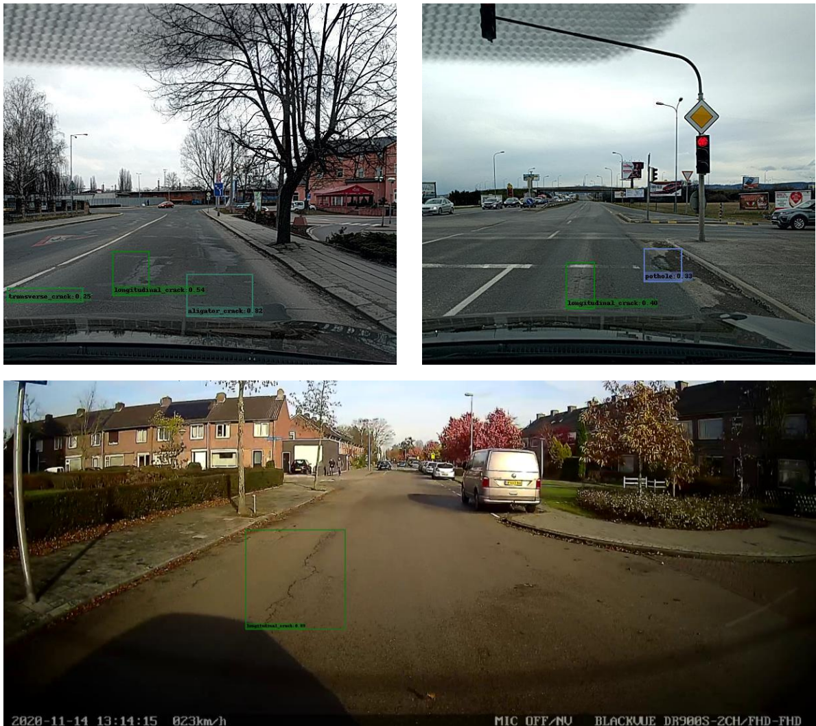
Figure 5: Examples of road damage detection using our detection model. The damages are marked with colored bounding boxes, with each color indicating a different type of damage.
