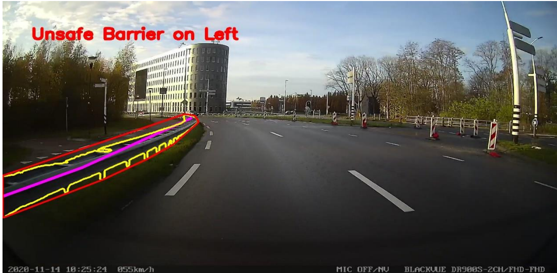
Figure 12: Example of barrier segmentation and barrier safety check.
